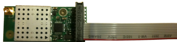
The cable attached to the CRMX™ OEM TRX
